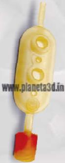
Eggshell rigid plastic to create sacrificial tooling that withstands silicone injection at high temperature and pressure, but breaks away easily. It shatter easily from silicone once the mold is filled and cooled. Its amber color allows for visualization of the injected silicone.
